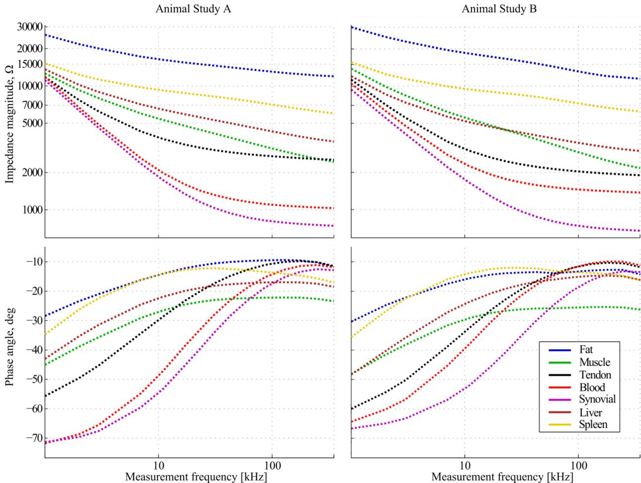
**Figure 4 - Mean impedance and phase angle spectra obtained in the two animal studies**
