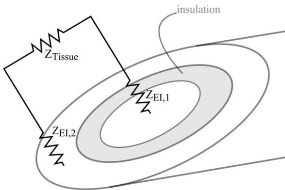
**Figure 2 - Bipolar impedance measurement using BIP Needle**
