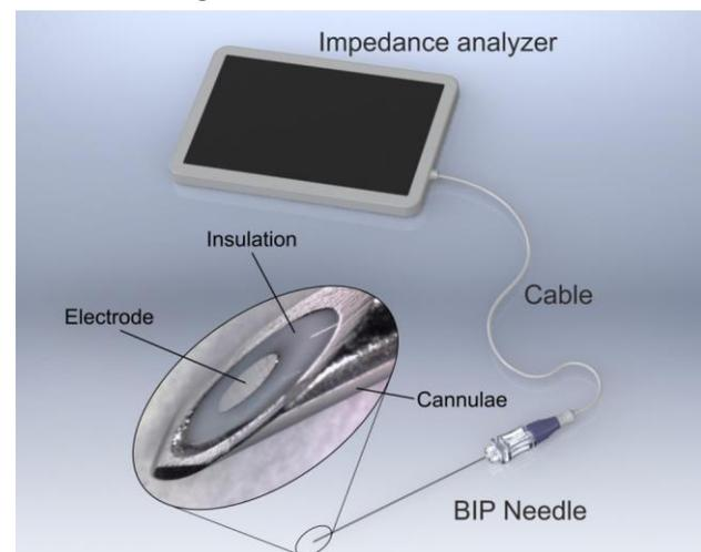
**Figure 1 - Illustration of the BIP Needle concept by Injeq Ltd**
