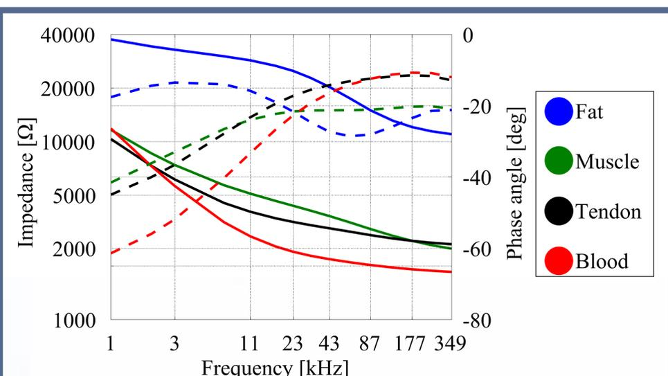
Figure 3: Average impedance magnitude (solid lines) and phase angle values (dashed lines) as a function of frequency
