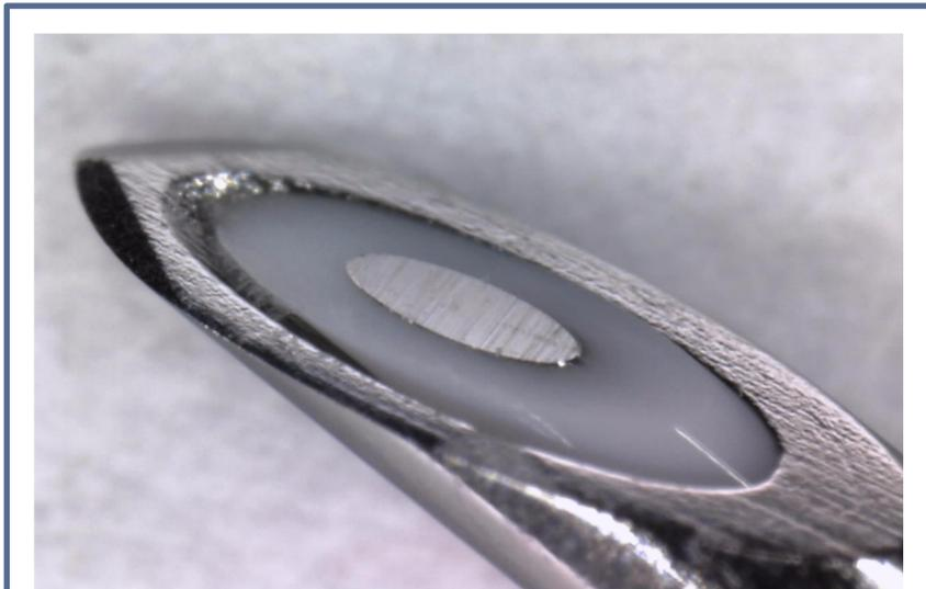
Figure 1: Bioimpedance probe (BIP) inside a standard 22 G spinal needle
