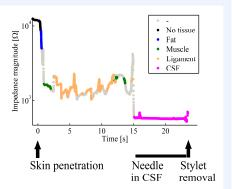
Example lumbar puncture. When needle tip gets in contact with CSF, device alerts physician. Single frequency data plotted.
